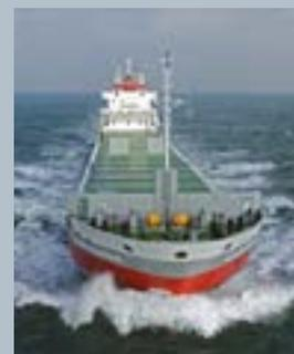
in terms of length, width or draft due to specific channels or locks. Take the EasyMax, for example: here we deliberately opted for a maximum draft of 8.60 metres, because this also allows the ship to navigate the Saint Lawrence and the Great Lakes on the other side of the Atlantic."
