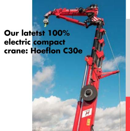
Wagenborg is continuously making her equipment more green. This applies not only to ships, but also to her equipment on land. For example, the fully electric Hoeflon C30e compact crane is a valuable addition to the existing crane fleet. Equipped with a 12 kW electric motor, the Hoeflon C30e has a maximum capacity of no less than 9,000 kg. The crane is very suitable for carrying out work in tight locations or in commercial buildings.
